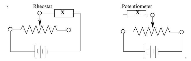
Physics labs often have large rheostats of assorted values of resistance and maximum current rating. These can be wired in either of the above configurations and are helpful in illustrating the role of resistors in series and parallel circuits. Illustrated below is the essential construction of two popular variable resistor configurations.
