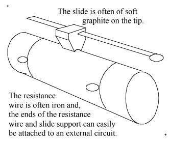
The shaft is attached to a sliding contact connected to the center tab.
