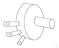
The two outside tabs are attached to either end of the resistance wire.
