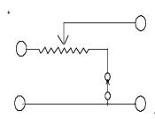
The voltage divider shown on the left is activated with the switch closed (down). The rheostat shown on the right is activated when the switch is opened (up).
