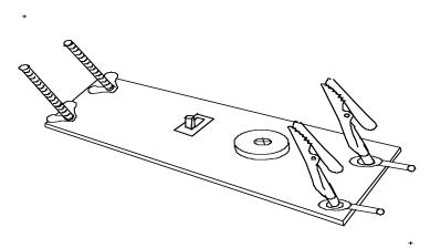
On the left is illustrated the low voltage device to reduce the output of the USB power source. The input is connected under the wing nuts on the far left. The output device to measure can be clipped in the alligator clips on the right. Under these clips are lugs to attach the probes of a voltmeter. The switch can change from a voltage divider to a rheostat configuration. The pot (potentiometer) is adjusted with a screwdriver.
