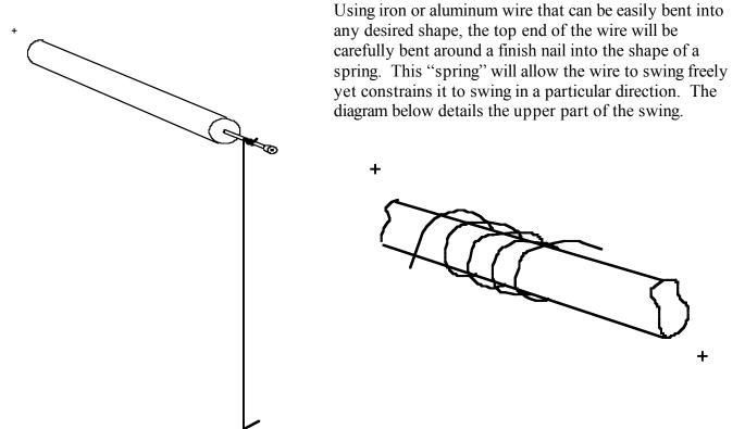
The lower end of this wire is bent at right angles so that as it swings, the suspended sphere will be released in the forward direction. As shown on the left, the finish nail is driven into a short length of dowel that can be supported with a ring stand.
