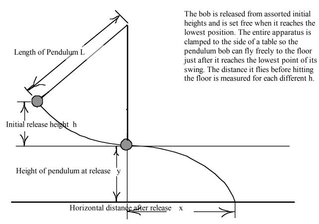
The pendulum bob should not be tied to the string, rather a special support is used that will hold the pendulum while it initially swings downward, but when the bob reaches its lowest position, the support will strike a stop block releasing the ball and allowing it to fly freely through the air.
