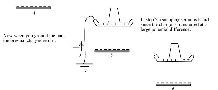
In step 6 the pie pan is now neutral and as you lower it, electrostatic induction will again separate the charges and you will be ready to repeat the cycle as you return to step 1.
