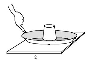
3. Remove your grounding finger and with your other hand, lift the pan by gripping the Styrofoam cup, to a distance of 10cm, or more, from the charged plate.
