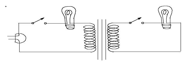
Initially both switches are closed and both bulbs are lit. Ask what will happen if the switch on the left is opened?
