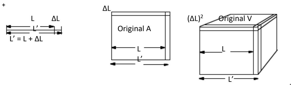
Note in the above illustration that when the area expands by  $\Delta L$  on a side, the area increases by  $2 \Delta L L$  and this is  $\Delta A$ . Hence  $A' = A + \Delta A = A + 2\alpha L^2\Delta T = A + 2\alpha A\Delta T$
