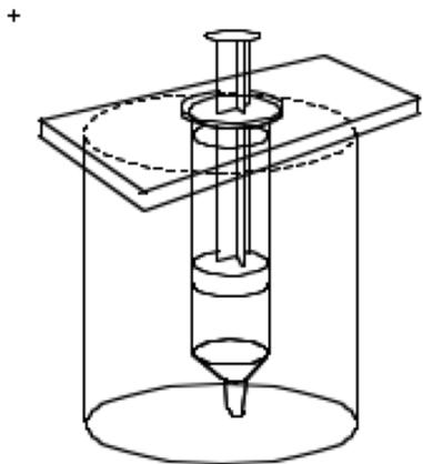
If a single board like the top board of the above structure is allowed to support the syringe, (shown on left) it can be lowered into several different large containers with different temperature water (ice, room, higher) to obtain constant pressure at different temperature for Charles' Law.
