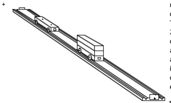
The track and carts illustrated on the left are made from inexpensive materials and are distributed every other year at the NPTW. The carts are made from identical pieces of 2X4 lumber, the track is from a 4 foot piece of 1 x 6 with V shaped grooves. lined with aluminum angle. The wheels are from Pitsco and two large opposing magnets are inserted in one end of the cart with Velcro on the other end for inelastic collisions. The entire apparatus costs less than \$20.
