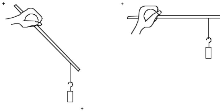
As shown on the left, first hold the large dowel with the weight downward. When the weight is all the way down, no torque is required but as it is rotated upward, more and more torque is required since the force is forming a more perpendicular angle with the moment arm.
