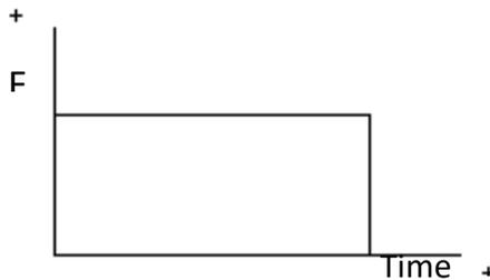
On the right is an impulse graph for a simple constant force. On the right is a more typical graph of impulse during a collision. The area under the graph is impulse.
