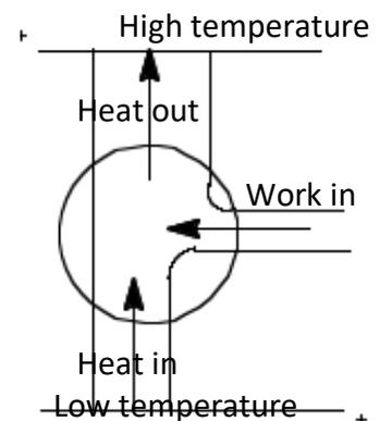
The circles in the diagrams above represent the systems using heat to produce work (heat engine) or using work to reverse the direction of heat flow (heat pump or refrigerator). More detailed PV diagrams can help to understand what is happening in actual systems. (A discussion of the typical internal combustion engine used in cars will be discussed on the next page.)
