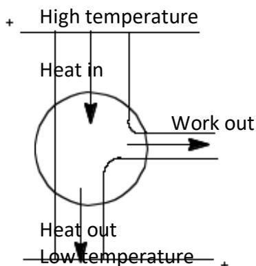
Typical schematic diagrams of heat engines (shown on the left) and heat pumps or refrigerators (shown on the right.) The 1<sup>st</sup> Law of thermodynamics describes the heat and work in and out of the system and the 2<sup>nd</sup> Law describes the direction of heat flow. If the refrigerator seems to violate the 2<sup>nd</sup> Law, remember that the work in also requires some sort of engine that will involve more, high to low heat transfer than the reverse by the refrigerator.
