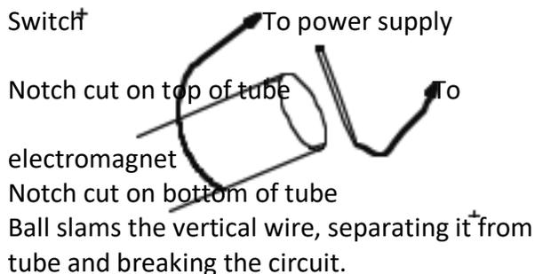
The gun consists of a metal tube with an inside diameter of about  $\frac{1}{2}$  “ that will freely accommodate a  $\frac{1}{2}$ ” steel ball. A simple switch (illustrated on the left) at the end of the tube is in series with a power supply and an electromagnet to hold up the target. The gun is firmly clamped and aimed at the target. The ball can be blown with sufficient strength to hit the target before both hit the floor.
