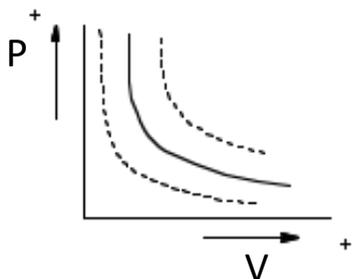
On the left is the pressure vs. volume graph for Boyle's law and on the right is the temperature vs. volume graph for Charles' law. The temperature vs. volume graph is a great way to extrapolate from "normal" temperatures to absolute zero.
