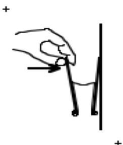
After establishing that equal and opposite forces are required to open the binder clip, have a single student press the clip against a wall to open it. It should be obvious that the wall presses back. On the right is shown the usual way to open the clip and it should also be obvious that equal and opposite forces are required. The same idea can be used with pulling forces and rubber bands.
