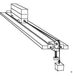
As an actual lab experiment, a horizontal distance along the track can be marked and measured, and then the time for the accelerating mass (from rest) can be measured for several runs. Using this time and distance the acceleration can be calculated. With the illustration on the right above, the acceleration should be: a = g/7. (The mass "m" falls out.) Depending upon the units used in the time and distance measurements, the acceleration can be computed in terms of g.
