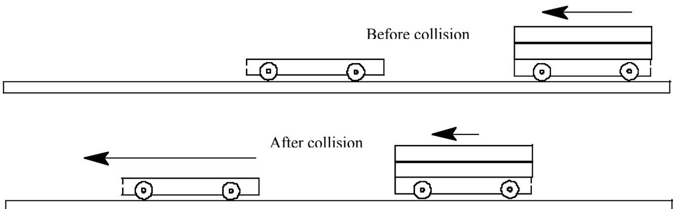
A qualitative discussion should lead to the conclusion that the loaded cart will not be able to “unload” all of its momentum before it comes to rest, hence must continue to move after the collision at a smaller velocity. The unloaded cart will move off at a much higher velocity.
