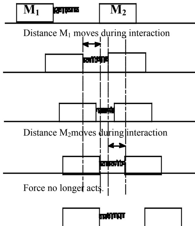
Momentum is always conserved since the force and time are the same no matter how far each object moves during the interaction. The elastic collision transfers both momentum and kinetic energy. The inelastic collision also observes momentum conservation but not kinetic energy conservation. It is also interesting to note that during the heart of the elastic collision, even kinetic energy is not conserved since some energy is temporarily stored in the spring as potential energy.
